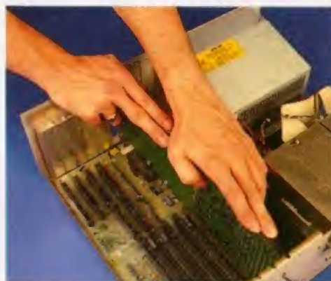
4 Fitting a Zorro card is easy. Just remove the blanking plate and slot it in. Press firmly on the card to make sure it fits properly in the connector.
